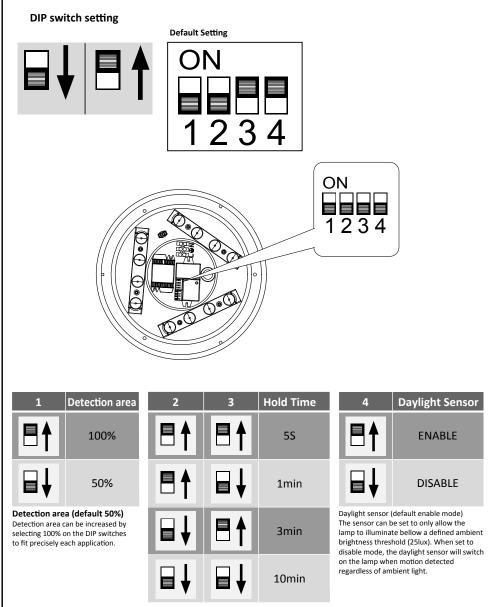
Hold time (default 3 min.) Refers to the time period the lamp remains at 100% illumination after no motion detected.
