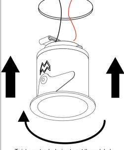
Twist counterclockwise to put through hole then twist clockwise to fixate
