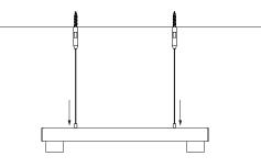
feed the cable into the lamp
