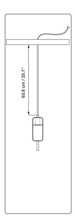
Hang canopy on to ceiling plate, securely installed into ceiling.
