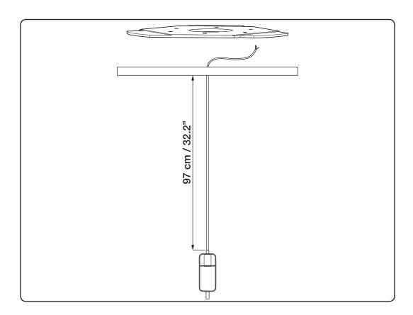
Pull the cord through the hole in the ceiling plate. The cord should measure about 97 cm - measured from the plate to the socket.
