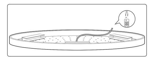
Connect the cord to the outlet in the ceiling.
